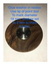
If you are going to make more than 1 set of these shakers you should make a drilling guide. Here is the way I made mine. I used a piece of hardwood that already had a tenon cut on one end, face off the other end if it needs it and mark the tenon diameter with the jig then hollow a recess out to the marked diameter, about 1/8" deep. Check to see if the
