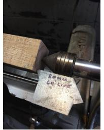
Mount your blank between centers and make a tenon on one end for your 50 mm chuck jaws. I use a marking device of my own design to mark the tenon diameter on the end of the turning blank. It is a piece of sheet metal that has been cut to make a point to
