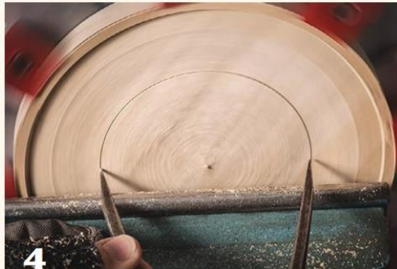
Making a 7½"-diameter plate, the author chooses his largest chuck jaws for remounting the work. Using dividers, he marks the necessary spigot, or tenon, size on the bottom of the plate.
