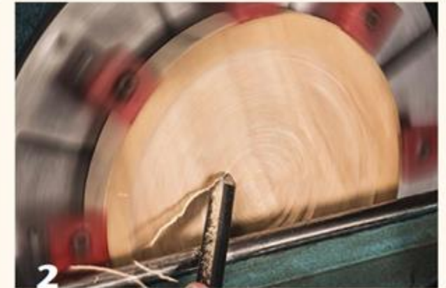
With a precut ¾"-thick blank mounted on bowl jaws, true the surface using a pull cut.
