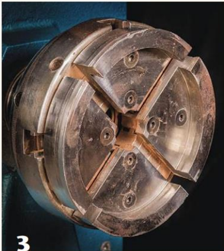
Making a 7½"-diameter plate, the author chooses his largest chuck jaws for remounting the work. Using dividers, he marks the necessary spigot, or tenon, size on the bottom of the plate.
