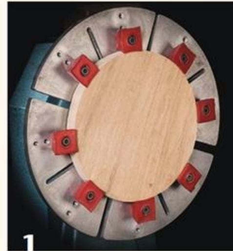
With a precut ¾"-thick blank mounted on bowl jaws, true the surface using a pull cut.
