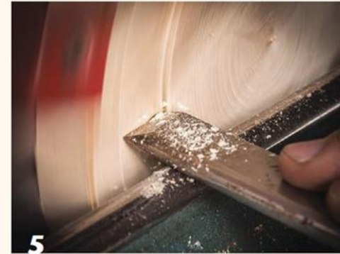
Using a skew chisel presented flat on the toolrest, the author forms a shallow spigot. Just \frac{1}{8} " depth is enough with a tenon this wide.
