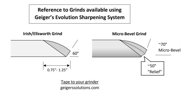
The above grinds are easily obtainable using the Evolution sharpening system.
