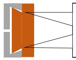
If the angle of the wooden dovetail doesn't match the angle of the chuck jaws, the ability to hold the blank securely is sacrificed.
