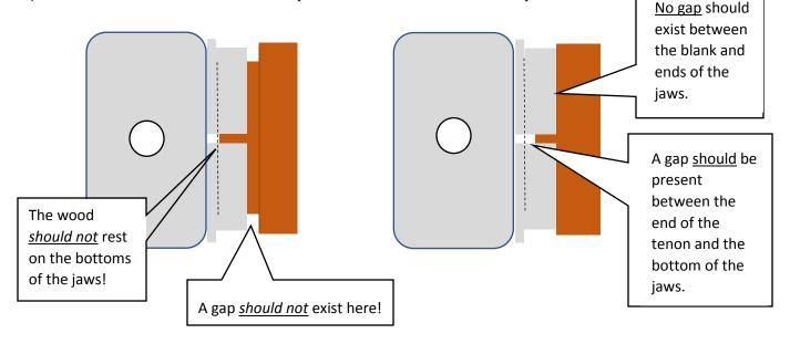
4) The angle of the wooden dovetail doesn't match the angle of the jaws.
