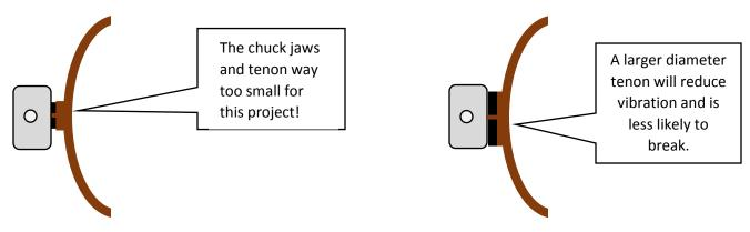
2) The turner produces a tenon too large in diameter to be safely held in the chuck jaws.
